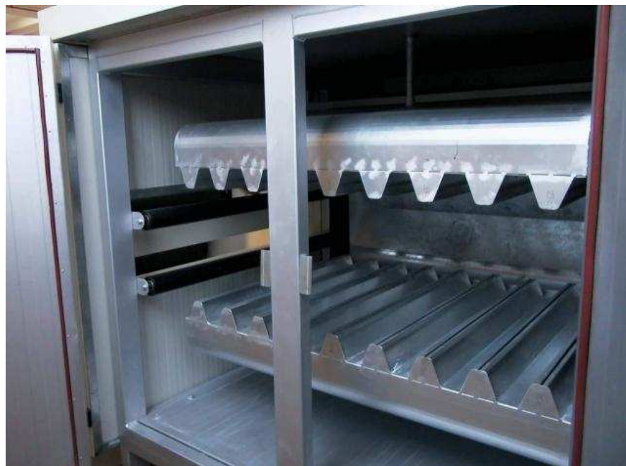
Air blades of drying oven
